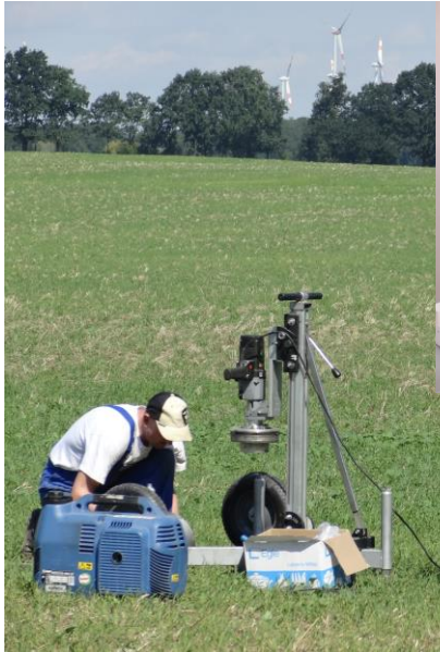
Sampling undisturbed soil cores
